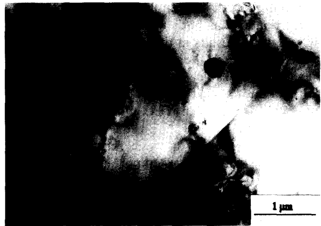
Fig. 3. The microstructure of \text{Al}_2\text{O}_3 -5 vol% SiC nano-composites, observed using TEM.
